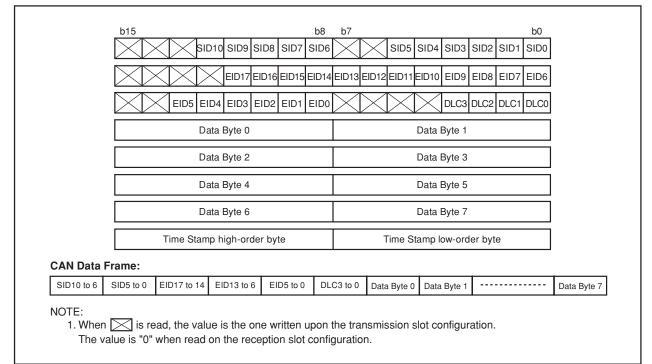
Figure 18.3 Bit Mapping in Word Access
